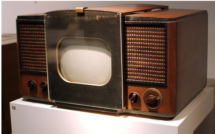
The RCA 630-TS, the first mass-produced television set, sold from 1946 to 1947.
