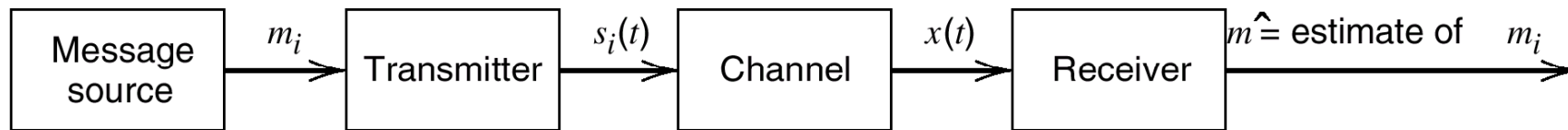
Figure 5.1 Block diagram of a generic digital communication system.
