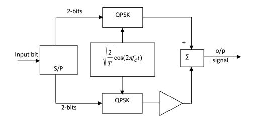
The above communication system transmits equally likely symbols each consists of 4-bits. An amplifier is inserted in the lower arm of Gain G=3 the input bit is in NRZ "L" with amplitudes  $\pm$  1 volts for digits 1 and 0, the bit duration is 1 sec. The noise
