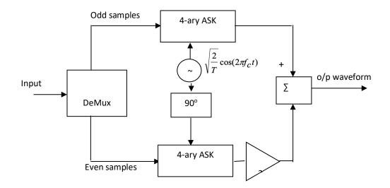
The above communication transmitter is used to emit one of 16 equally likely messages over AWGN channel with zero mean and two sided PSD= 1 w/Hz. The quantizers used in the 4-ary ASK modulators are mid-riser with output  $\pm \frac{a}{2}$ ,  $\pm \frac{3a}{2}$ . An amplifier of gain = 2 is inserted in the lower arm. Assuming the o/p symbol duration T= 2 Sec. a = 2 volts and  $f_c = 100.25$ Hz.
