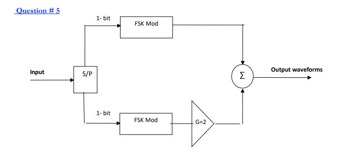
The above Tx consists of two identical CBFSK modulators. An amplifier of Gain G=2 is inserted in the lower arm, then the outputs the two arms are added coherently to form the output waveform.
